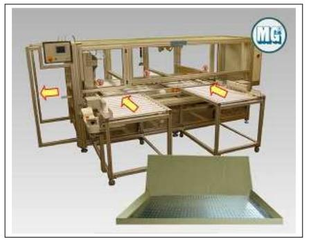
Stapling large packages up to 4 layers of double wall corrugated cardboard (wrap around cartons for packing steel sheets).
